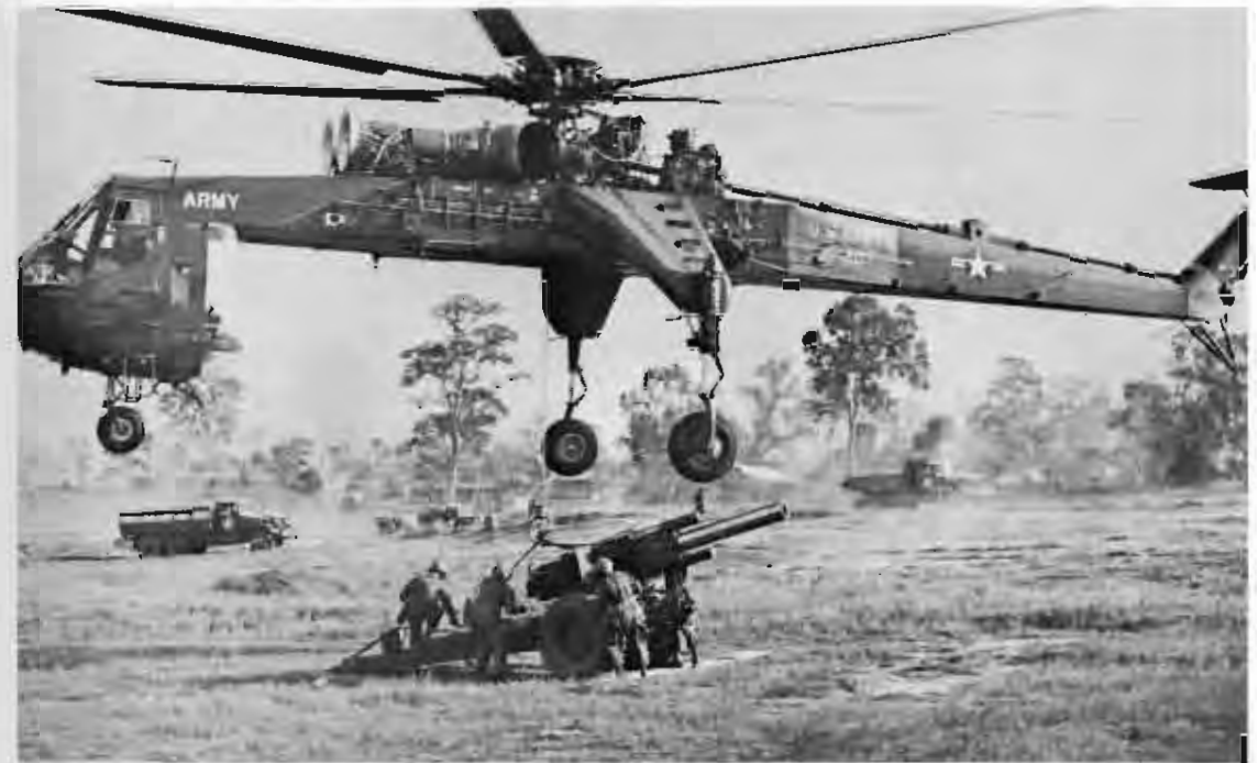
CH-54 SKYCRANE emplacing 8" howitzer
